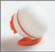
150021 Camping Lantern Bulb:3 W LEDs Luminous: high mode: 60-65Lm Low mode::20Lm Size:62x53mm Weight:96g Colour:Available color Battery:rechargeable With micro USB cable Function50% on/100% on/flash /off Power indicator and Hook Magnetic Bottom Waterproof: IP 43 Lighting Memory Function
