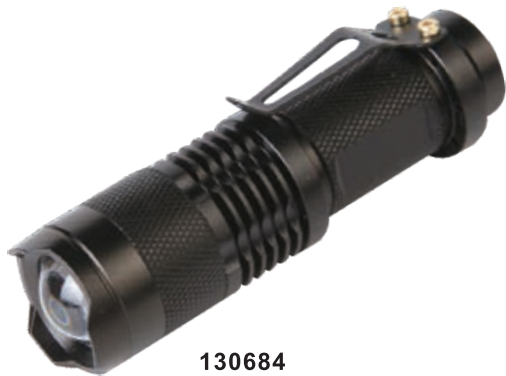
130684 Material:Aircraft-grade Aluminium Bulb:CREE Q5(150LM) Battery: 1x14500 Function:high/low/flash Telescopic focus,water-resistant and with clip
