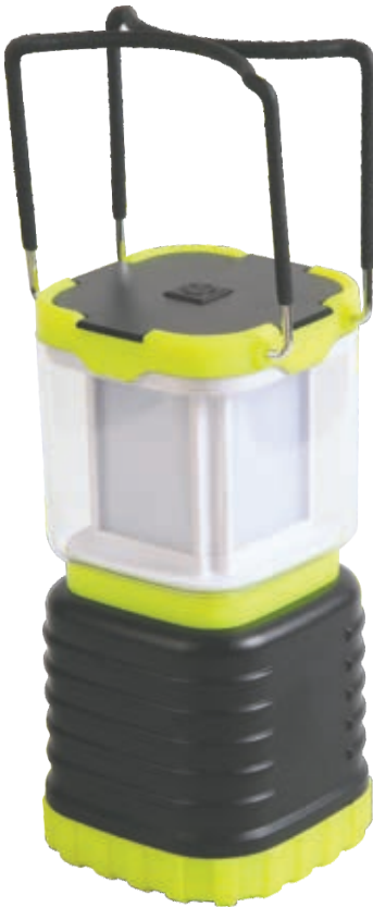
150039 Camping lantern Size:90×90×182mm Material:ABS/GPPS Bulb:16 white LEDs(LED paster:0.5w) Battery: 3.7V/3600MAH rechargeable Li-ion battery With one USB/MICR05P(80cm) USB transformer not included Function:100% on/50% on/off
