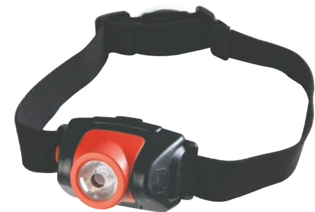
160011 T1249 LED headlamp light color:white ,red, green,blue Headband color:black battery:3xAAA with push-button switch water proof: Ip44 Headband Length:50-60cm headband width:2.5cm 120 lumens initial brightness headlights Headlight headlight features: 100% On - 50% on 25% off bright -SOS- Headlight taillight features: bright - flash - off
