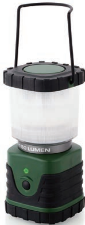
120019 Multi-functional camping lantern. middle size Bulb: 1W/3W CREE LED(150 Lumen / 300 Lumen) Battery: 3D Function: 50% on/100% on/Flash/off The lantern can hanged upside down after cover taken. Easy-find green light blinks every 5 seconds when light is in off position.
