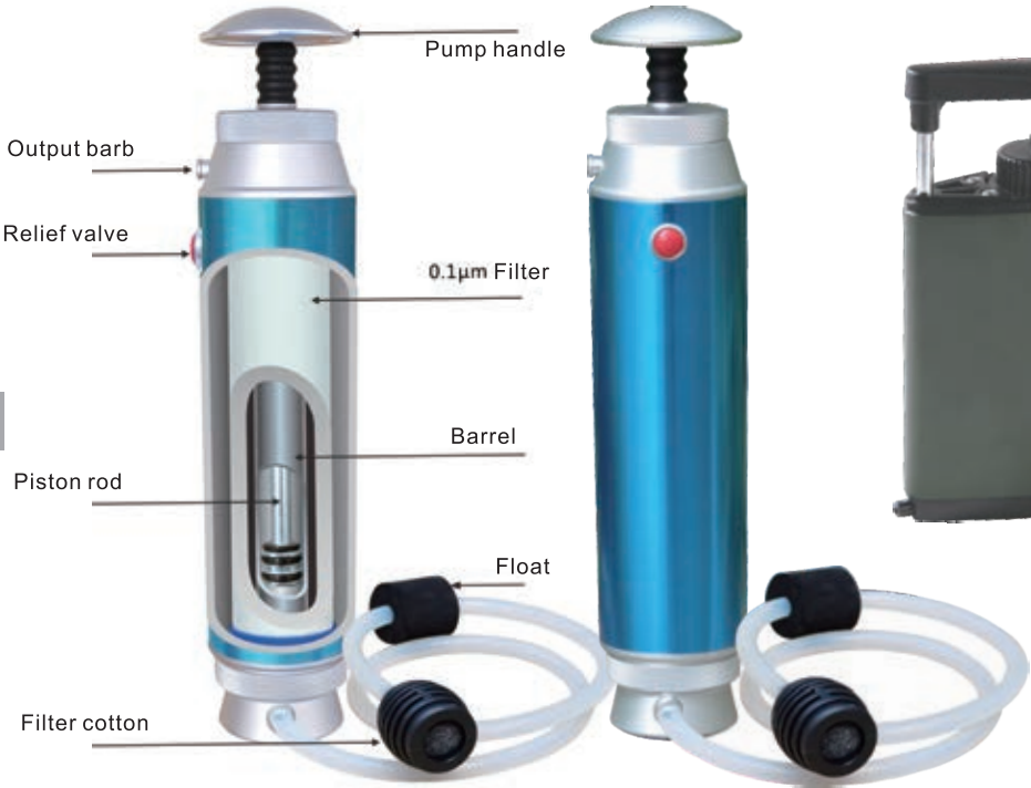
140082 Portable water filter bottle Size: 78x265mm, 3000L, 195g All kinds of fresh water can be used. Applicable for hiking, camping, fishing and climbing, emergency relief support. Pocket water microfilter Material: Antibacterial GAC, ABS, AL, silica, ceramic Size: 47x220mm, 53000L, 455g All kinds of fresh water can be used. Applicable for hiking, camping, fishing and climbing, emergency relief support. Portable, small and compact, durable.
